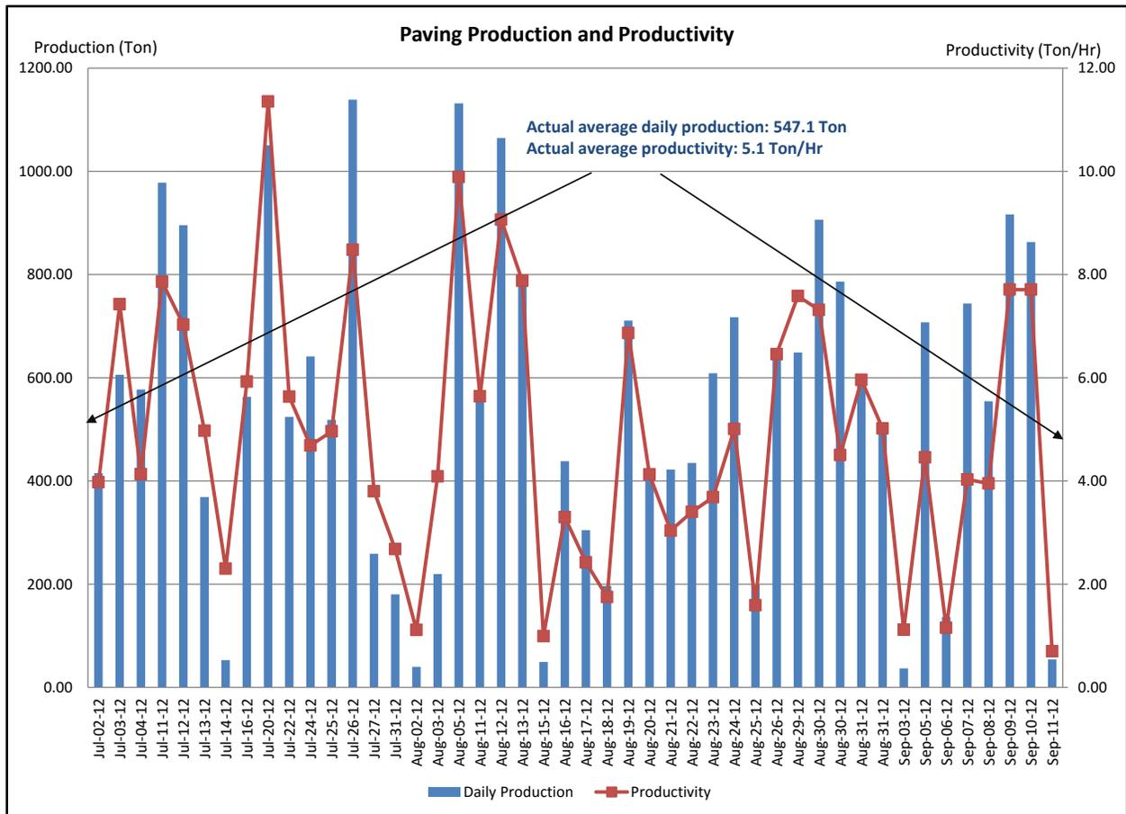
Figure 2 – Case Study 1: Paving Productivity on the Non-Zero Production Days
